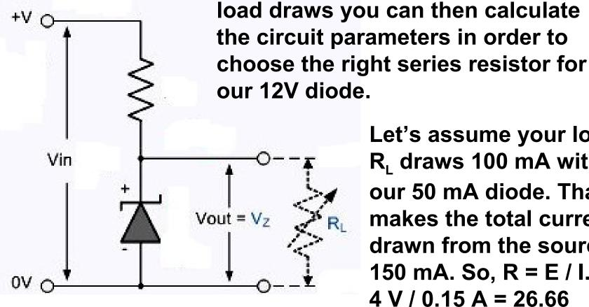
Let's assume your load R<sub>1</sub> draws 100 mA with our 50 mA diode. That makes the total current drawn from the source 150 mA. So, R = E / I. 4 V / 0.15 A = 26.66 ohms.
