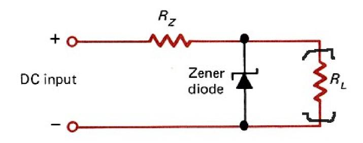
Here's the Zener diode connected as a so-called "shunt regulator."
